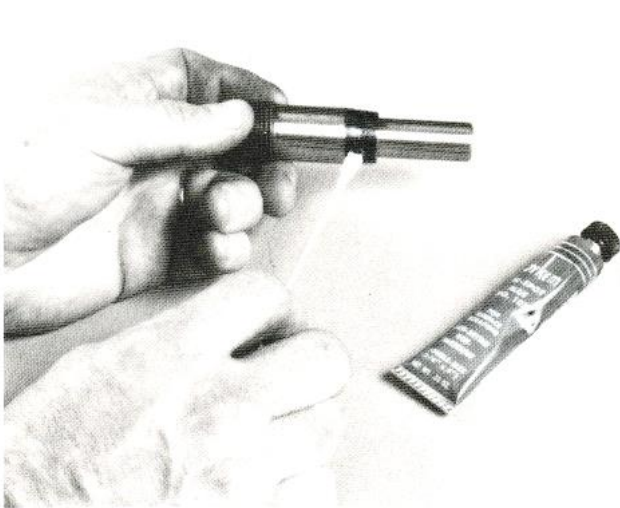
Step 1 Deposit Hi Spot Blue on taper portion of the taper locating screw.
