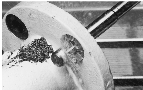
Spindle with coolant through (CT).
