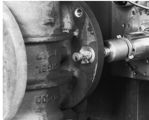
Back spotfacing large valve body.
