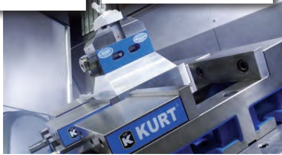
MaxLock 5 axis vise mounted in a Kurt vise used as a receiver.
