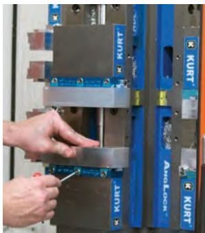
DoveLock jaws provide 1 minute changeover
