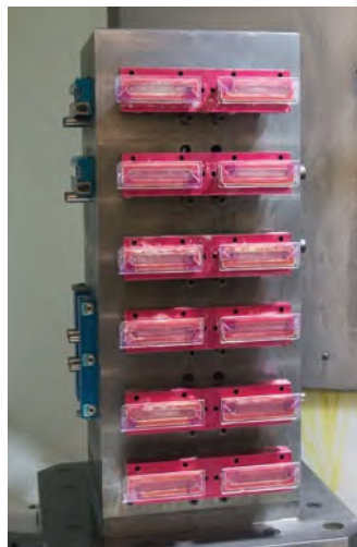
DoveLock jaws used for glass machining
