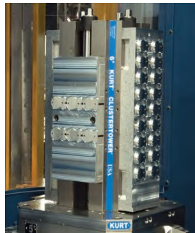
Cluster Tower using fixture plate & Soft jaws
